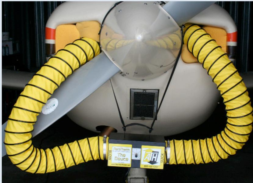
suspension band that allows the unit to hang from the prop of your aircraft, carrying tubes and four sponges to seal the engine inlets. It's portable enough to take with you. Unfortunately, it lasted only one season for me but in all fairness, I have no idea how long it had been in service or how it had been used or treated by its previous owner. I was completely satisfied with the Classic's
