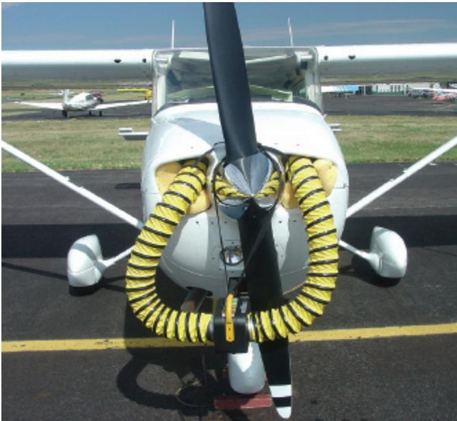
engine components to the same temperature. This is important because airplanes utilize cast iron engine cylinders, and the cast iron should be the same temperature as the aluminum pistons. Uneven heating of the pistons results in piston scoring, which occurs when the pistons are hotter than the engine cylinder. This problem is typical of oil heaters which also cause condensation due to uneven heating.
