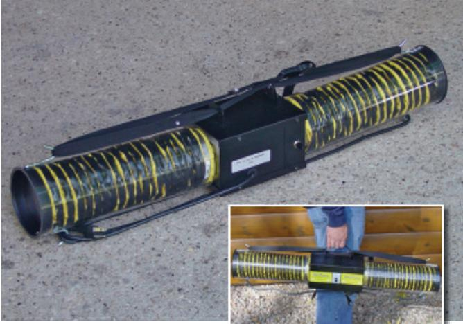
When packed in the portable carrying case, the AeroTherm Deuce measures 38.25" x 6.5" x 7" and weighs 11 pounds.
